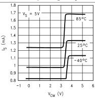
Figure 9.  $I_S$  vs.  $V_{CM}$
