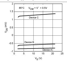
Figure 5.  $V_{OS}$  vs.  $V_{S}$  for 3 Representative Units
