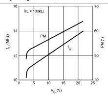
Figure 17. Unity Gain Freq. and Phase Margin vs. V<sub>S</sub>
