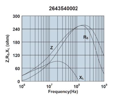
Impedance, reactance, and resistance vs. frequency.
