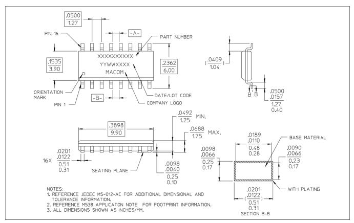
t Reference Application Note M538 for lead-free solder reflow recommendations. Plating is 100% matte tin over copper.
