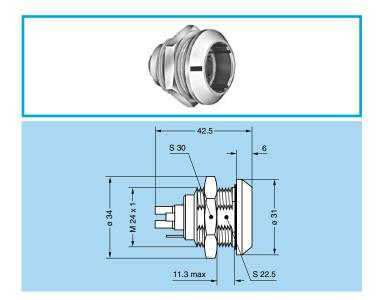
ENW.3K Fixed socket, nut fixing, keys (W), and earthing tag
