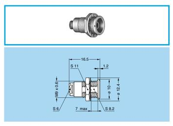
EEG.0B Fixed active device housing, nut fixing, key (G) or keys (A...F), (back panel mounting)
