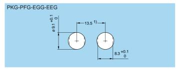
Note: ¹) Minimum distance between two neighbouring components. Mounting nut torque: 2.5 Nm. The value shown above is the maximum torque for each connector type.
