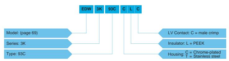
**EDW.3K.93C.CLC** = Fixed socket with rear square flange, keys (W), 3K series, mixed type to accept 2 F2 type fibre optic contacts, 2 power and 2 signal electrical contacts, chrome-plated brass housing, PEEK insulator, male crimp signal contacts.
