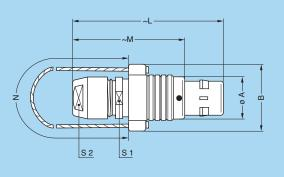
FNG Straight plug, key (G) or keys (A...L and R) and cable collet with lanyard release
