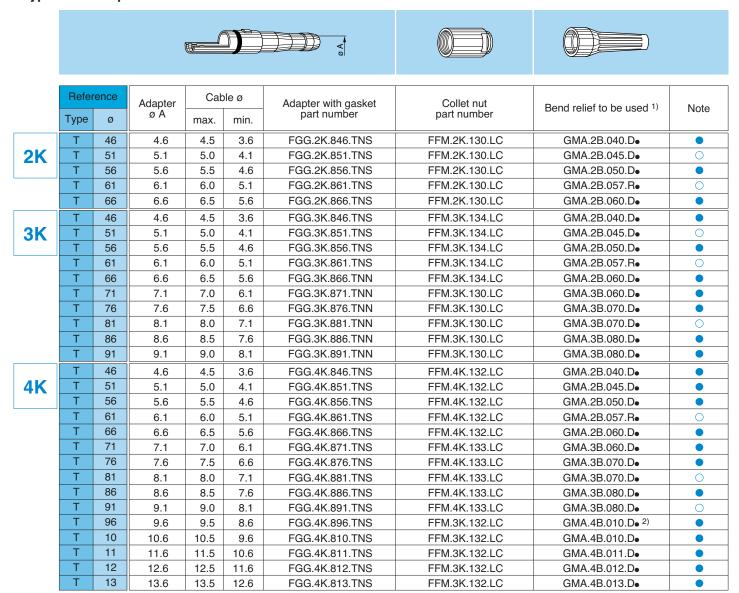
Note: 1) The bend relief is to be ordered separately (see pages 91 and 92). 2) Add a short piece of heat-shrink tubing under the bend relief.
