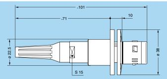
FMW.3K Fixed plug with round flange (4 holes fixing), keys (W), cable adapter, with bend relief
