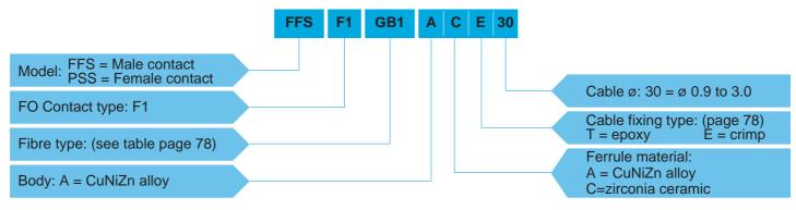
**FFS.F1.GB1.ACE30** = Male F1 type fibre optic contact, ferrule bore diameter of 235 μm, ferrule made of zirconia ceramic, crimp type cable fixing for a cable diameter of 0.9 mm to 3.0 mm.
