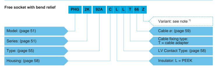
**PHG.2K.92A.CLLT66Z** = Free socket with key (G), 2K series, mixed type to accept 1 F2 type fibre optic contact and 2 low voltage contacts, chrome-plated brass housing, PEEK insulator, 2 female solder electrical contacts, cable fixing type T for 6.5 mm diameter cable, and nut for fitting a bend relief.
