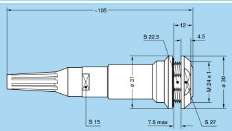
PEW.3K Fixed socket, nut fixing, keys (W), cable adapter, with bend relief (back panel mounting)
