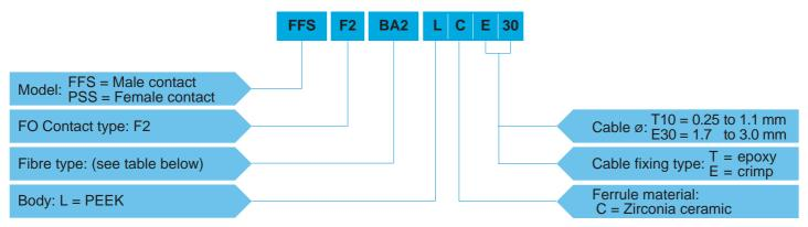
**FFS.F2.BA2.LCE30** = Male F2 type fibre optic contact, ferrule bore diameter of 125  $\mu$ m, PEEK body, Zirconia ceramic ferrule, crimp cable fixing, for tight jacket cable with a diameter between 1.7 to 3.0 mm.
