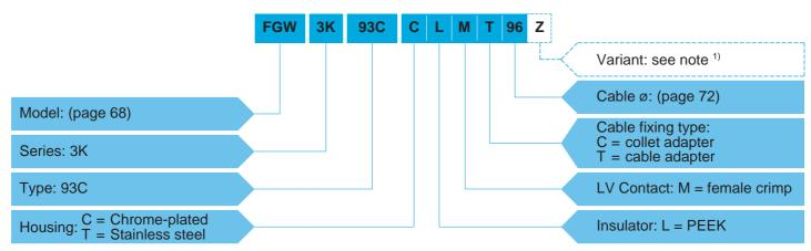
**FGW.3K.93C.CLMT96Z** = Straight plug with keys (W), 3K series, mixed type to accept 2 F2 type fibre optic contacts, 2 power and 2 signal electrical contacts, chrome-plated brass housing, PEEK insulator, female crimp signal contacts, cable fixing type T for 9.2 mm diameter cable, and nut for fitting a bend relief.
