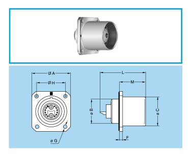
EDG Fixed socket with square flange, key (G) or keys (A...F, L and R), protruding shell and earthing tag, screw fixing
