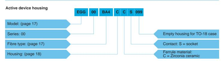
**EGG.00.BA4.CCS099** = Straight active device housing, nut fixing with key (G), 00 series, with ferrule for F4 fibre optic contact, assembled with single-mode fibre  $\emptyset$  9/125, chrome-plated brass housing, zirconia ceramic ferrule, socket contact, empty housing for TO-18 case.
