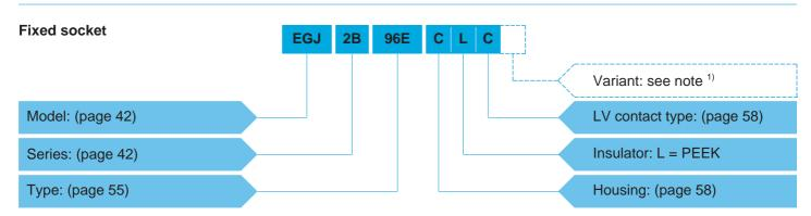
**EGJ.2B.96E.CLC** = Fixed socket with key (code J) 2B series, mixed type to accept 1 F1 fibre optic contact and 6 low voltage electrical contacts, chrome-plated brass housing, PEEK insulator, 6 male crimp electrical contacts.
