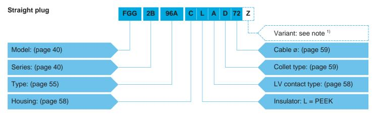
**FGG.2B.96A.CLAD72Z** = Straight plug with key (G), 2B series, mixed type to accept 1 F1 fibre optic contact and 2 low voltage electrical contacts, chrome-plated brass housing, PEEK insulator, 2 male solder electrical contacts, type D collet system to suit a 7.2 mm diameter cable, and a nut for fitting a bend relief.
