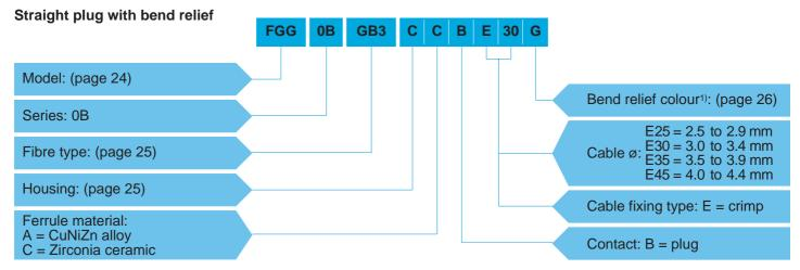
**FGG.0B.GB3.CCBE30G** = Straight plug with key (G), 0B series, F3 fibre optic contact, ferrule hole diameter 235  $\mu$ m, chrome-plated brass housing, zirconia ceramic ferrule, plug type contact, crimp type cable fixing for 3.0 to 3.4 mm diameter cable, and gray bend relief.
