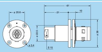
FXW.3K Fixed plug with round flange (4 holes fixing), keys (W)
