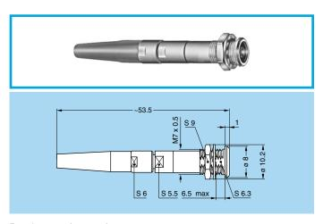
PEG.00 Fixed socket, nut fixing, key (G) or key (B), with bend relief (back panel mounting)
