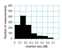
Mean = 0.25 dBTested at 1300 nm Tested according to the standard IEC 61300-03-04, Insertion Method B. Fibre =  $50/125 \mu m$ Ferrule bore diameter = 126 µm
