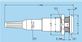
PKG Fixed socket, nut fixing, key (G) or keys (A...F, L and R) and cable adapter and nut for fitting a bend relief
