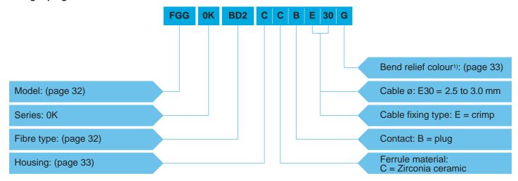
**FGG.0K.BD2.CCBE30G** = Straight plug with key (G), 0K series, F2 fibre optic contact, ferrule hole  $\emptyset$  128  $\mu$ m, chrome-plated brass housing, zirconia ceramic ferrule, plug type contact, crimp type cable fixing for 2.5 to 3.0 mm diameter cable, and gray bend relief.
