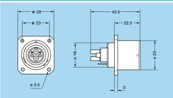
EDW.3K Fixed socket with rear square flange (4 holes fixing), keys (W), and earthing tag
