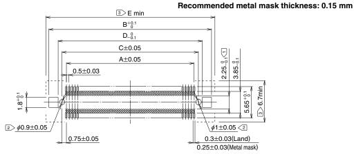
Note 1 The cross-hatched area inside the SMT land may come into contact with the connector contacts and thus care should be taken that the pattern does not extend beyond the SMT land width.
