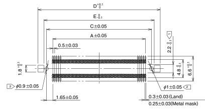
Note 1) The cross-hatched area 🖾 inside the SMT land may come into contact with the connector contacts and thus care should be taken that the pattern does not extend beyond the SMT land width. 2) Not required in products without guideposts.
