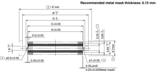
Note 1) The cross-hatched area 🖾 inside the SMT land may come into contact with the connector contacts and thus care should be taken that the pattern does not extend beyond the SMT land width.
