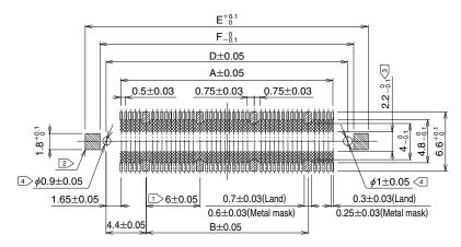
Note  $\boxed{1}$  Cross-hatched portions, totaling n places, indicate the ground circuits.
