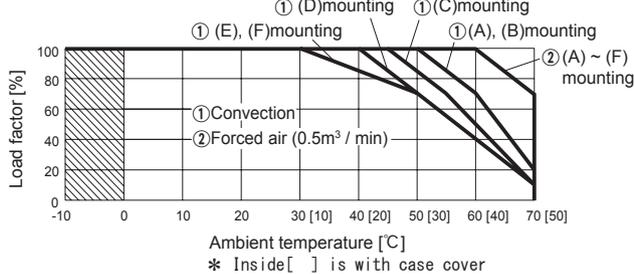
● LFA100F Ambient temperature derating curve (Reference value)
