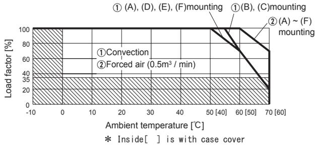
● LFA15F Ambient temperature derating curve (Reference value)
