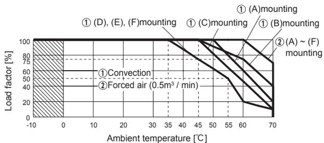
● LFA100F-□-SN Ambient temperature derating curve (Reference value)
