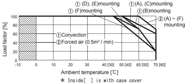
● LFA50F Ambient temperature derating curve (Reference value)
