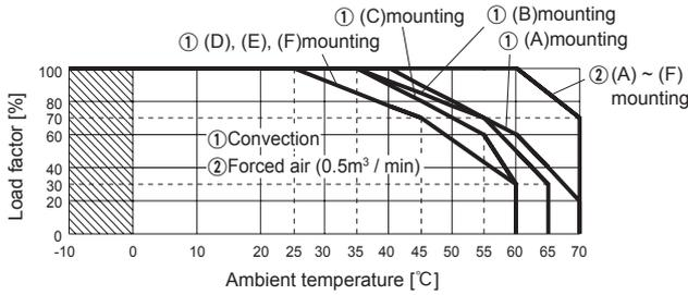
● LFA150F-□-SN Ambient temperature derating curve (Reference value)
