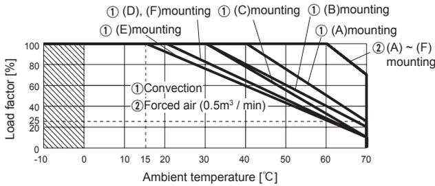
● LFA240F-□-SN Ambient temperature derating curve (Reference value)
