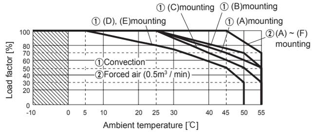
● LFA240F Ambient temperature derating curve (Reference value)
