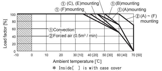
● LFA75F Ambient temperature derating curve (Reference value)
