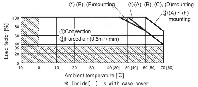
● LFA30F Ambient temperature derating curve (Reference value)
