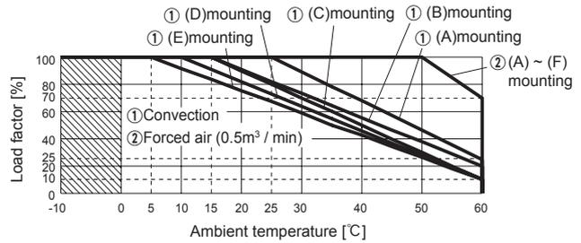
● LFA300F Ambient temperature derating curve (Reference value)
