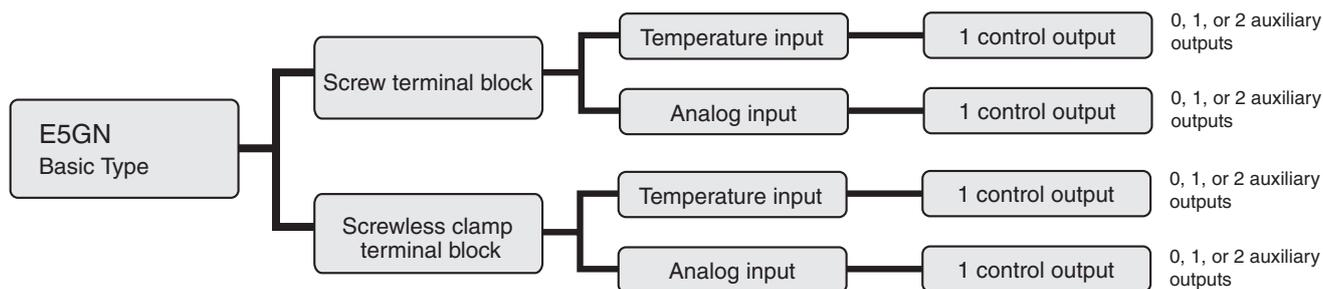
**Note:** Models with one control output and one or two auxiliary outputs can be used for heating/cooling control.
