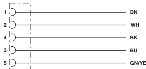
Contact assignment of the M12 sockets
