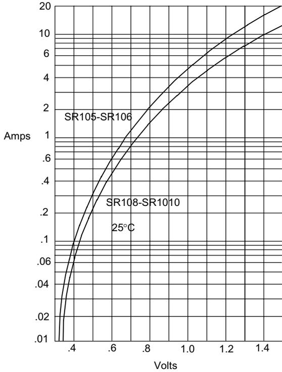
Instantaneous Forward Current - Amperes versus
