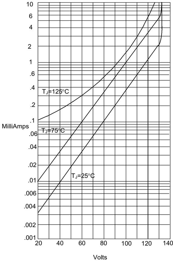
Instantaneous Reverse Leakage Current - MicroAmperes versus
