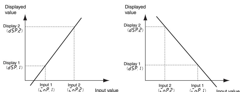
Instead of setting by inputting with the Shift Key and Up Key, current measurement values can be input as scaling input values for teaching. This is useful for making settings while checking the operation status of the K3GN.
