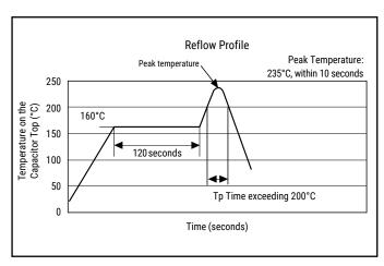
Above "Reflow Profile" graph indicates temperature at the terminals and capacitor top.
