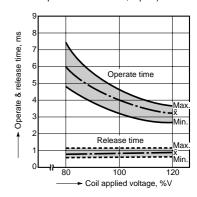
4.-(4) Operate & release time (with diode, 1 Form A)
