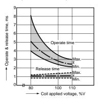
4.-(3) Operate & release time (without diode, 2 Form A)
