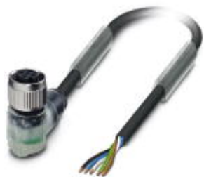
Sensor/actuator cable, 5-position, Variable cable type, free cable end, on Socket angled M12 SPEEDCON, A-coded, with 3 LEDs, cable length: Free input (0.2 ... 40.0 m)
