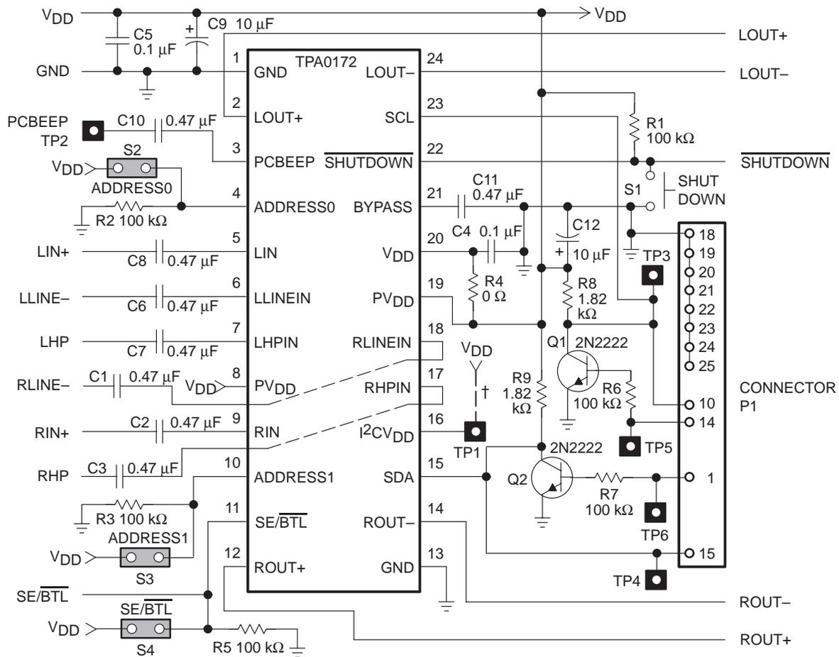
† I<sup>2</sup>CV<sub>DD</sub> is connected to V<sub>DD</sub> via a blue wire on the evaluation module. To use a different voltage for the I<sup>2</sup>C interface, the wire must be disconnected and the I<sup>2</sup>C power supply connected to TP1.
