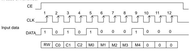
(Note3) In case of over than 12 bits data, valid data is the first 4 bits as System control data and the last 8 bits as Timer data. (In case of Days of week, it is the last 4 bits is effective.)
