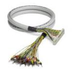
Round cable assembled with a 20-pos. socket strip and an open end. On the open end, the wires are labeled with 1 to 20 and have ferrules, cable length: 10 m
