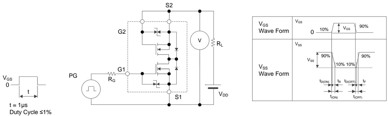
Test Circuit 8  $t_{D(ON)}$ ,  $t_R$ ,  $t_{D(OFF)}$ ,  $t_F$
