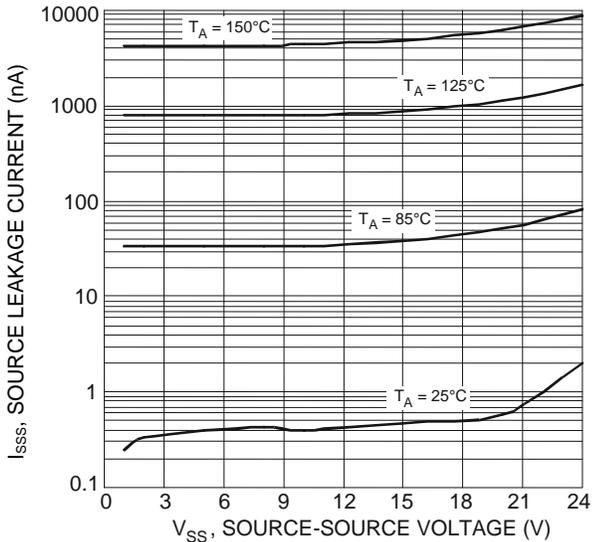
Figure 9. Typical Source-Source Leakage Current vs. Voltage
