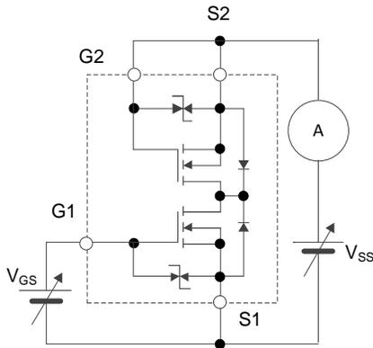
Test Circuit 3  $V_{GS(OFF)}$
