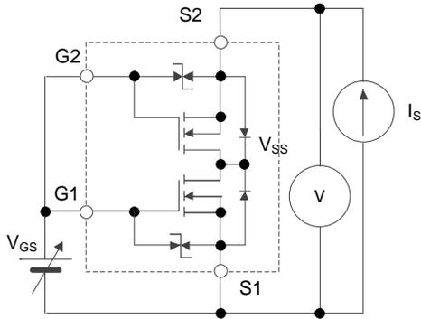
Test Circuit 5  $R_{SS(ON)}$
