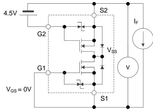
Test Circuit 6  $V_{F(S-S)}$
