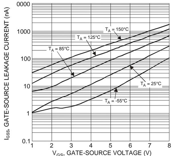
Figure 10. Typical Gate-Source Leakage Current vs. Gate-Source Voltage
