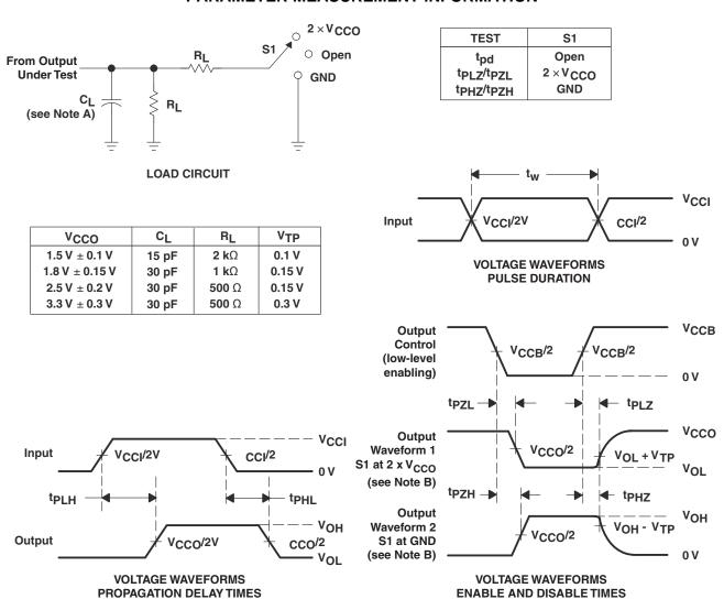
Figure 2. Load Circuit and Voltage Waveforms
