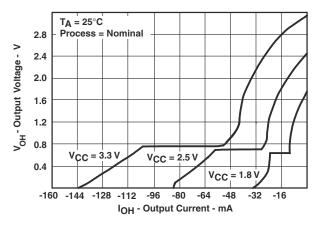
Figure 1. Typical Output Voltage vs Output Current
