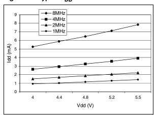
Figure 62. Typical I<sub>DD</sub> in SLOW mode
