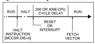
Figure 28. HALT Mode Flow-chart
