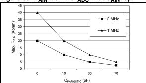
Figure 84. Recommended C<sub>AIN</sub> & R<sub>AIN values.</sub><sup>2)</sup>
