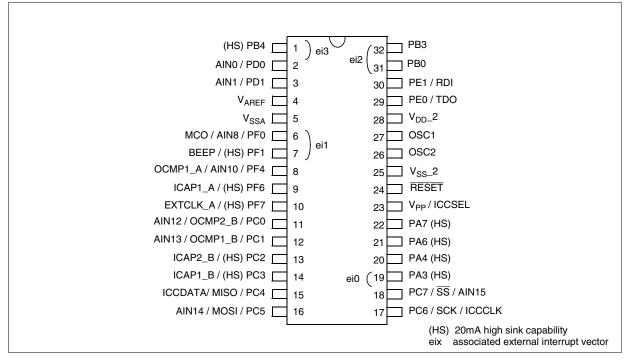
Figure 4. 32-Pin TQFP 7x7 Package Pinout
