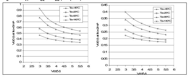
Figure 75. Typical V<sub>OL</sub> vs. V<sub>DD</sub> (high-sink ports)
