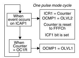
Then, on a valid event on the ICAP1 pin, the counter is initialized to FFFCh and OLVL2 bit is loaded on the OCMP1 pin, the ICF1 bit is set and the value FFFDh is loaded in the IC1R register.
