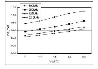
Figure 63. Typical I<sub>DD</sub> in WAIT mode
