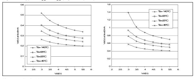
Figure 76. Typical  $V_{OH}$  vs.  $V_{DD}$
