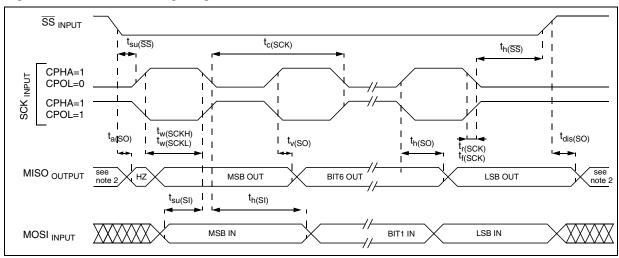
Figure 82. SPI Master Timing Diagram 1)
