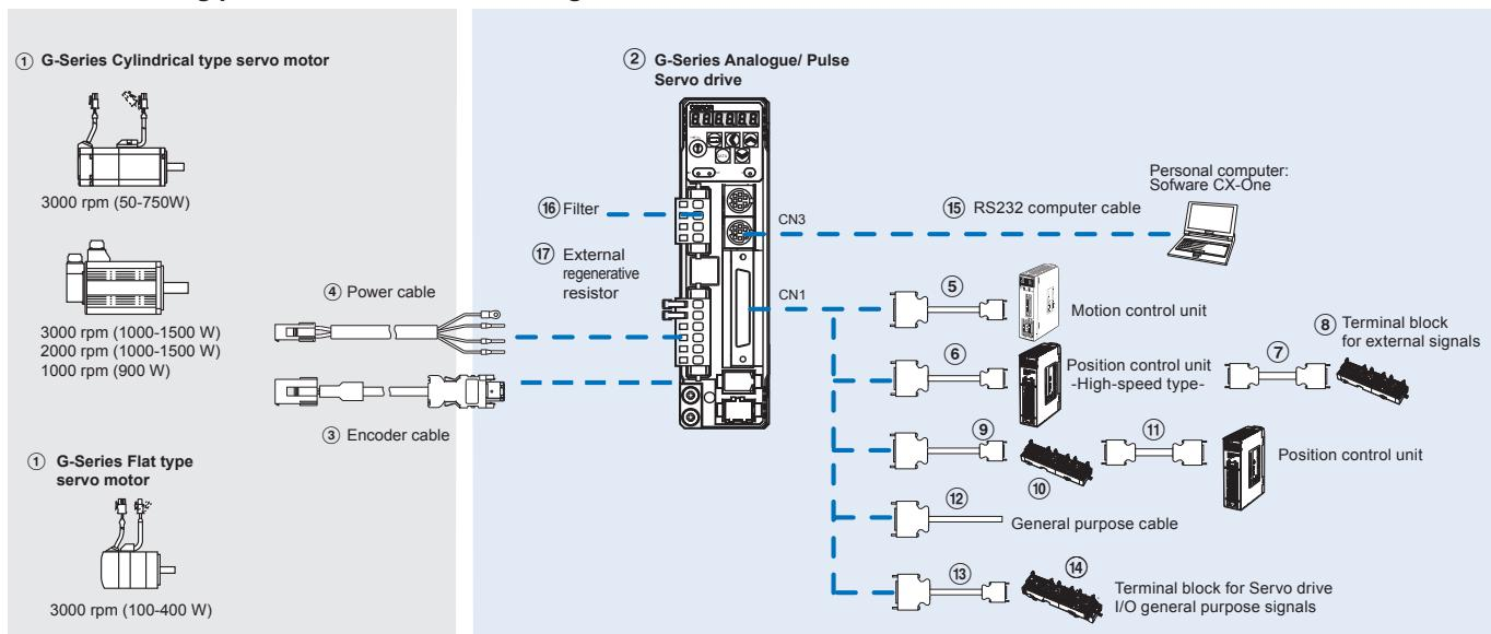
**Note:** The symbols ①②③④⑤... show the recommended sequence to select the components in a G-Series servo system
