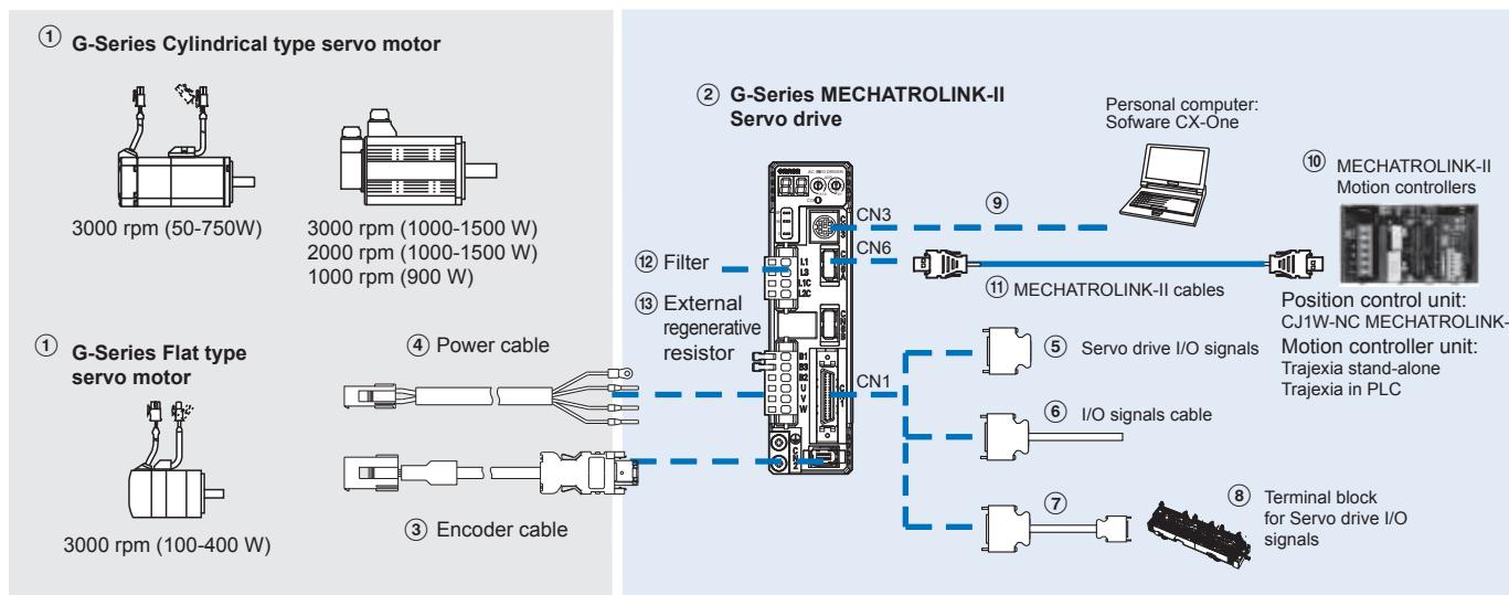
Note: The symbols ① ② ③ ④ ⑤... show the recommended sequence to select the components in a G-Series servo system
