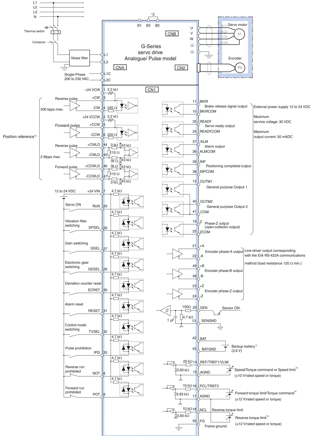
\*1 For use only with an absolute encoder. If a backup battery is connected to CN1 I/O connector, an encoder cable with a battery is not required.
