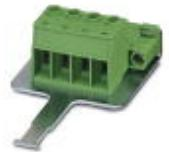
Plug component, Nominal current: 76 A, Rated voltage (III/2): 1000 V, Number of positions: 3, Pitch: 10.16 mm, Connection method: Screw connection with tension sleeve, Color: green, Contact surface: Silver
