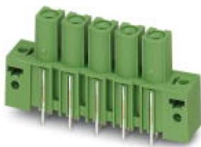
Header, Nominal current: 76 A, Rated voltage (III/2): 1000 V, Number of positions: 3, Pitch: 10.16 mm, Color: green, Contact surface: Silver, Mounting: Wave soldering
