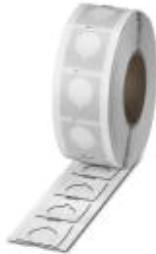
Plastic label with drill hole, Roll, white, unlabeled, can be labeled with: THERMOMARK ROLL 2.0, THERMOMARK ROLL, THERMOMARK ROLL X1, THERMOMARK ROLMASTER 300/600, THERMOMARK X1.2, mounting type: adhesive, lettering field size: 45 x 10 mm
