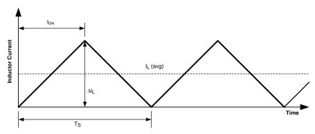
**Figure 13. Inductor Current Waveform**
