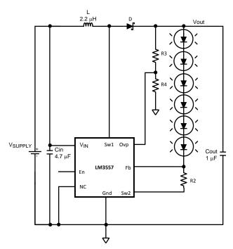
Figure 12. Programmable Output Voltage
