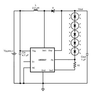
Figure 1. Backlight Configuration
