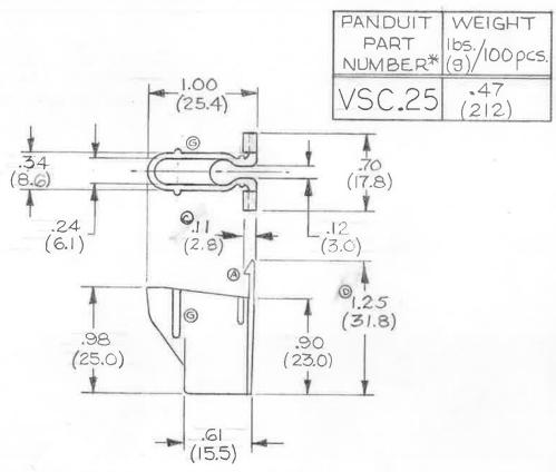
\*I, SEE CURRENT PRICE SHEET FOR PART NUMBER SUFFIX DESIGNATION FOR PACKAGE SIZE AND PART COLOR. 2. DESIGNED FOR USE ON ALUMINUM AND STEEL SIDING WITH THE PITTSBURGH INTERLOCK TYPE LAP JOINT.
