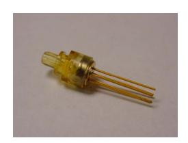
The HFD3141-203 use a high-performance InGaAs PIN photo-detector packaged with a transimpedance amplifier designed to meet performance requirements for data rates up to 4.25Gbps data communication over single-mode optical fiber at 1200nm to 1600nm. Applications include Ethernet, Fiber Channel and ATM protocols. The PIN is RoHS compliant per Directive 2011/65/EU<sup>1</sup>.
