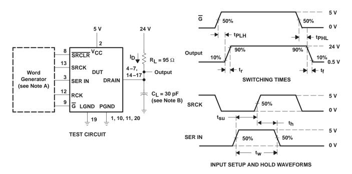
Figure 2. Test Circuit, Switching Times, and Voltage Waveforms
