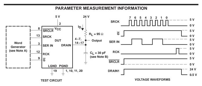
Figure 1. Resistive Load Operation
