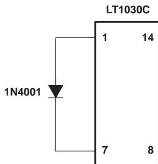
Figure 11. Connecting a Diode From  $V_{CC-}$  to GND
