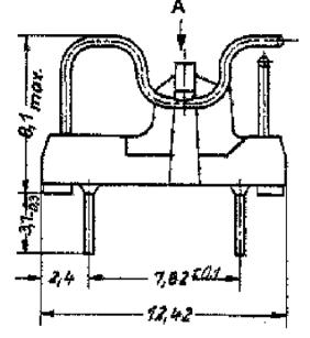
Sallbruchstellen, einzelne Verbindungen abtrennbar Predetermined breaking point, single connection units could be broken off
