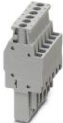
Plug, Connection method: Screw connection, Number of positions: 5, Cross section: 0.14 mm<sup>2</sup> - 4 mm<sup>2</sup>, AWG: 26 - 12, Width: 26 mm, Height: 47 mm, Color: gray
