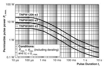
Maximum Pulse Load  $P_{i, max.}$  for Single Pulses
