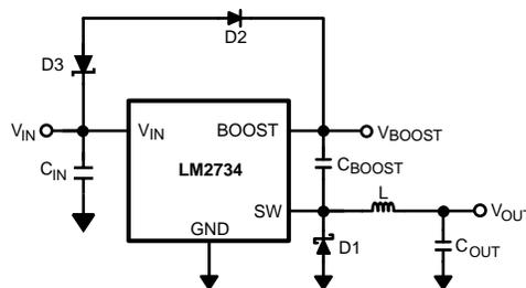
**Figure 14. Zener Reduces Boost Voltage from  $V_{IN}$**
