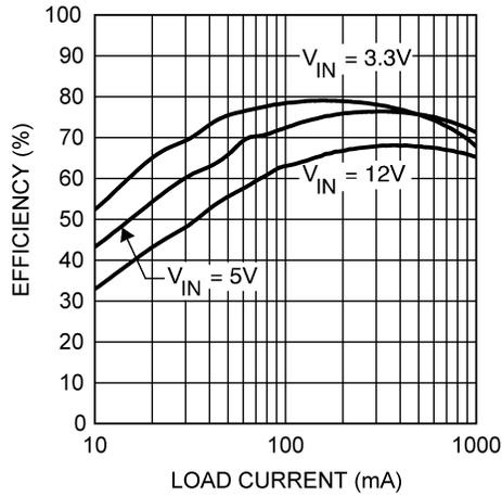
**Figure 21. Efficiency vs Load Current - L1 = 4.7 μH V<sub>OUT</sub> = 1.5 V**
