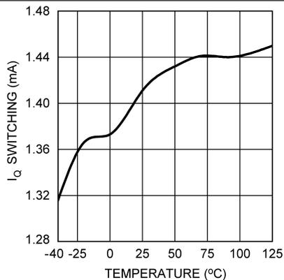
Figure 7. I<sub>Q</sub> Switching vs Temperature
