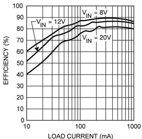
Figure 17. Efficiency vs Load Current - L1 = 4.7 μH V<sub>OUT</sub> = 5 V
