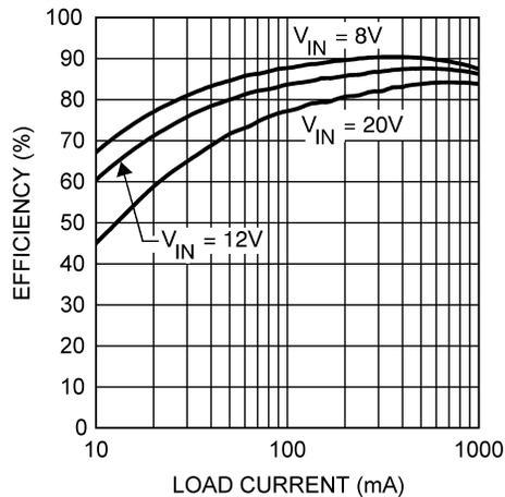
Figure 18. Efficiency vs Load Current - L1 = 10 μH V<sub>OUT</sub> = 5 V
