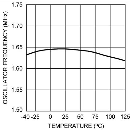
Figure 1. Oscillator Frequency vs Temperature - L1 = 4.7  $\mu\text{H}$
