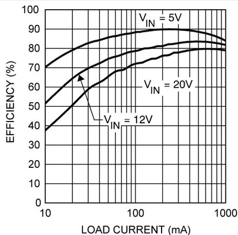
Figure 20. Efficiency vs Load Current - L1 = 10 μH V<sub>OUT</sub> = 3.3 V
