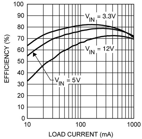
**Figure 22. Efficiency vs Load Current - L1 = 10 μH V<sub>OUT</sub> = 1.5 V**
