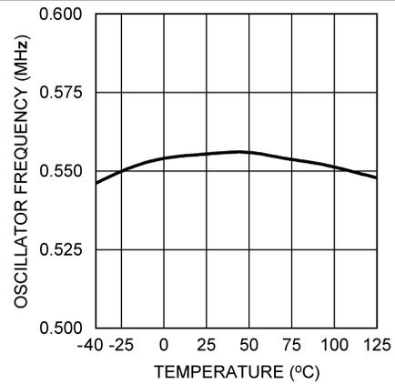
Figure 2. Oscillator Frequency vs Temperature - L1 = 10  $\mu\text{H}$
