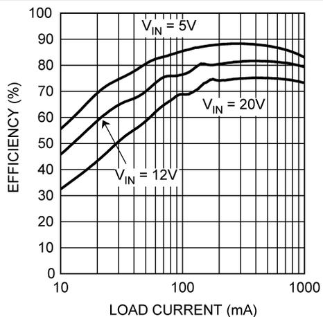
Figure 19. Efficiency vs Load Current - L1 = 4.7 μH V<sub>OUT</sub> = 3.3 V
