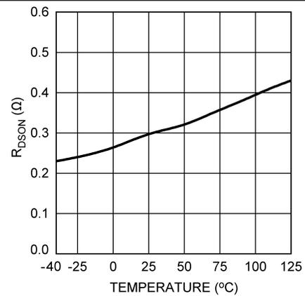
Figure 6.  $R_{DS(on)}$  vs Temperature
