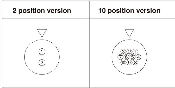
Note : The numbering of the contact is from the plug termination side.
