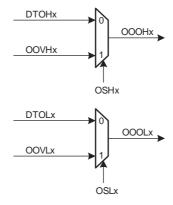
The fields OSHx and OSLx in the "PWM Output Selection Register" (PWM\_OS) allow the outputs of the dead-time generator DTOHx and DTOLx to be overridden by the value defined in the fields OOVHx and OOVLx in the "PWM Output Override Value Register" (PWM\_OOV).
