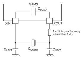
$C_{LEXT} = 2 \times (C_{CRYSTAL} - C_{LOAD} - C_{PCB})$
