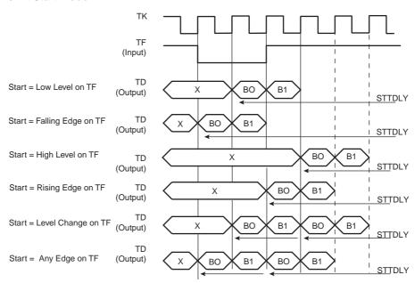
Figure 29-11. Receive Pulse/Edge Start Modes
