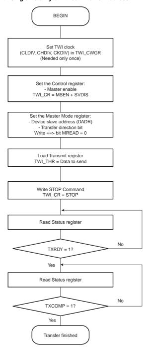
Figure 30-16. TWI Write Operation with Single Data Byte and Internal Address
