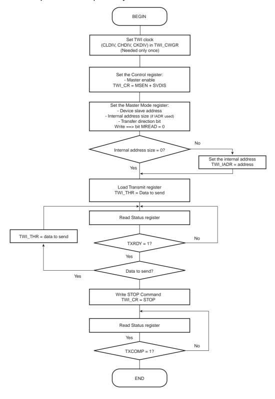
Figure 30-18. TWI Read Operation with Single Data Byte without Internal Address
