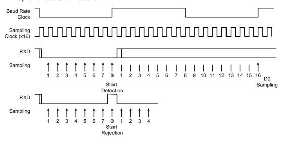
Figure 33-13. Asynchronous Character Reception
