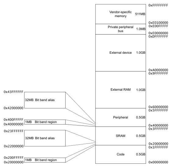
The regions for SRAM and peripherals include bit-band regions. Bit-banding provides atomic operations to bit data, see "Bit-banding" on page 54.
