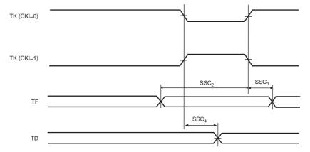
Figure 41-27. SSC Transmitter, TK and TF as Input
