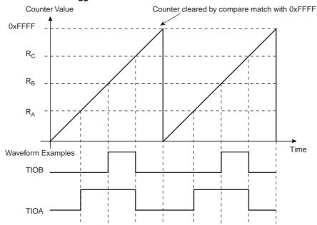
Figure 34-8. WAVSEL= 00 with trigger
