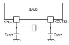
$$C_{LEXT} = 2 x (C_{CRYSTAL} - C_{para} - C_{PCB}).$$
