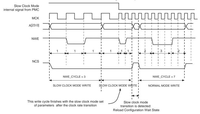
Figure 23-30. Recommended Procedure to Switch from Slow Clock Mode to Normal Mode or from Normal Mode to Slow Clock Mode
