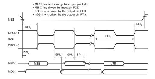
Figure 41-36. USART SPI Slave Mode (Mode 1 or 2)
