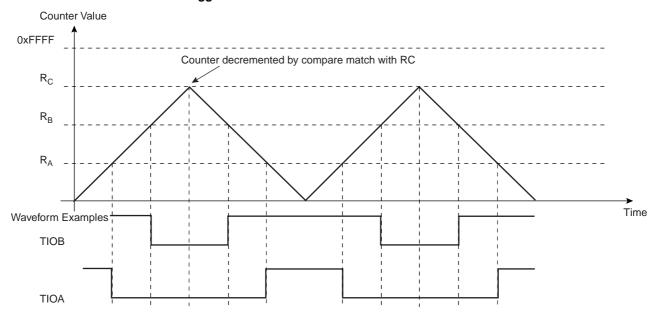
Figure 34-14. WAVSEL = 11 With Trigger
