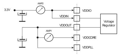
Figure 41-9. Active Mode Measurement Setup for VDDCORE at 1.62V
