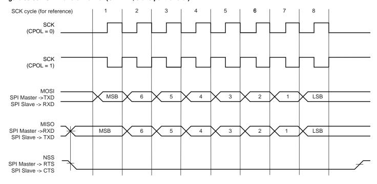
Figure 33-39. SPI Transfer Format (CPHA=0, 8 bits per transfer)
