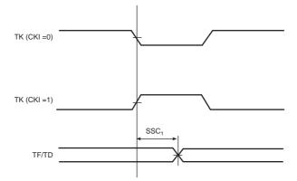
Figure 41-26. SSC Transmitter, TK as Output and TF as Input
