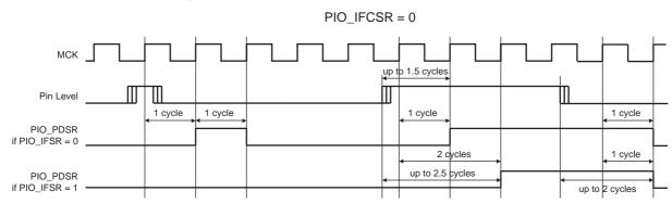
Figure 28-6. Input Debouncing Filter Timing
