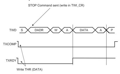
Figure 30-7. Master Write with Multiple Data Bytes
