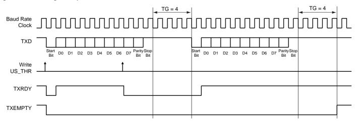
Table 33-10 indicates the maximum length of a timeguard period that the transmitter can handle in relation to the function of the Baud Rate.
