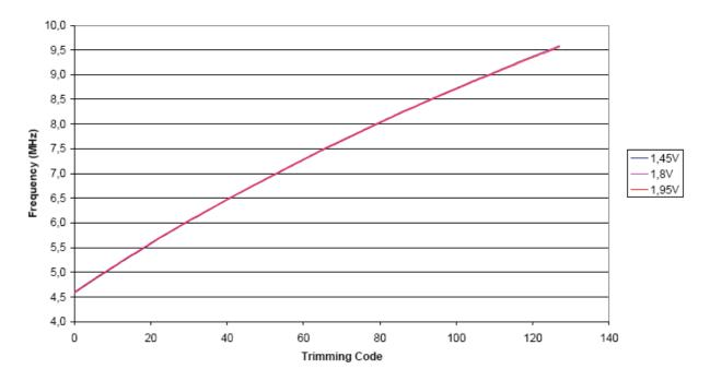
Figure 41-13. RC 12 MHz Trimming
