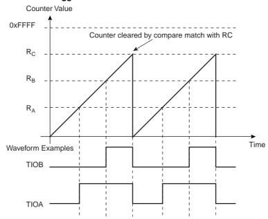
Figure 34-10. WAVSEL = 10 With Trigger
