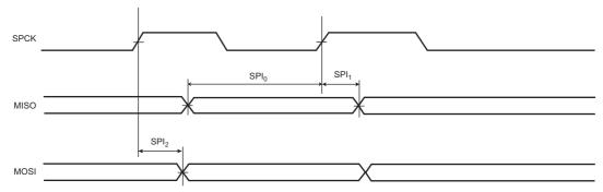
Figure 41-21. SPI Master Mode with (CPOL = 0 and NCPHA = 1) or (CPOL = 1 and NCPHA = 0)
