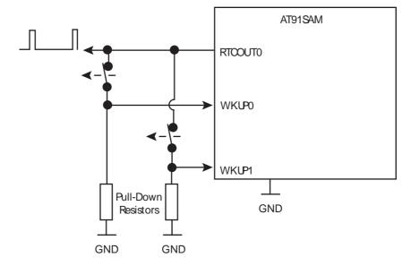
The debouncing parameters can be adjusted and are shared (except the wake up input polarity) by both debouncers. The number of successive identical samples to wake up the core can be configured from 2 up to 8 in the LPDBC field of SUPC\_WUMR. The period of time between 2 samples can be configured by programming the TPERIOD field in the RTC\_MR register.
