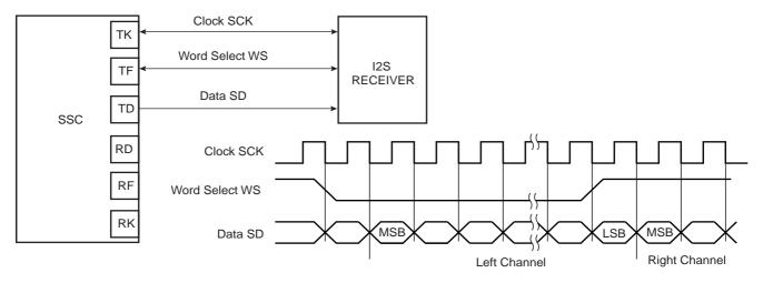
Figure 29-18. Codec Application Block Diagram
