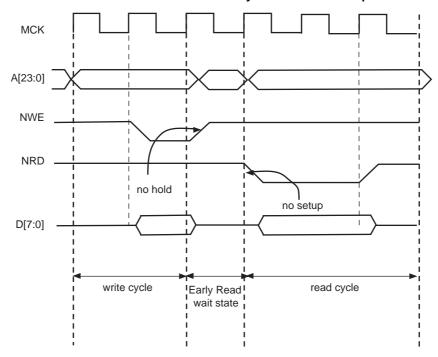
Figure 23-15. Early Read Wait State: NCS Controlled Write with No Hold Followed by a Read with No NCS Setup
