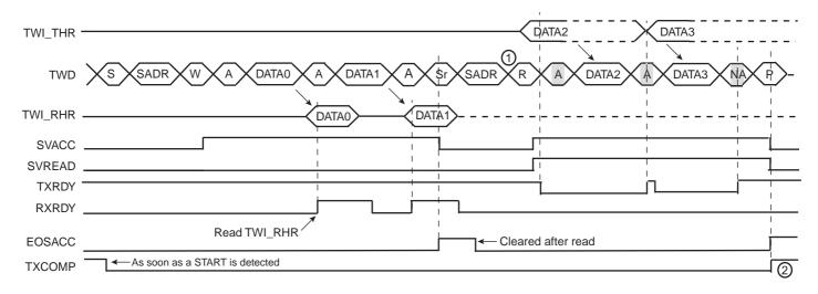
Notes: 1. In this case, if TWI\_THR has not been written at the end of the read command, the clock is automatically stretched before
