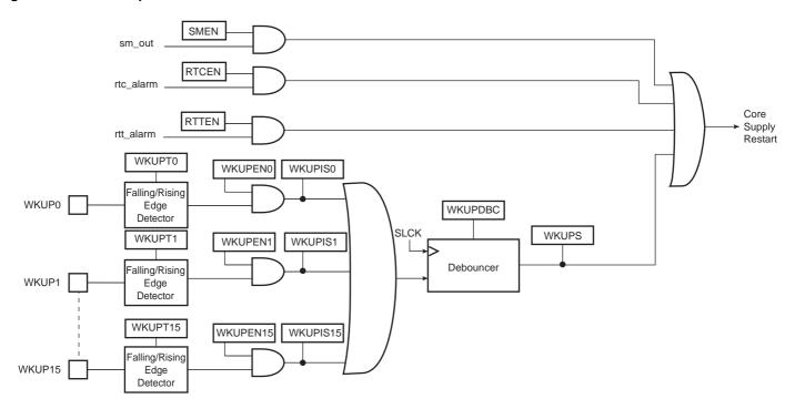
Note: Before instructing the system to enter Backup mode, if the field WKUPDBC > 0, ensure that none of the WKUPx pins that are enabled for a wake-up (exit from Backup mode) hold an active polarity. This is checked by reading the pin status in the PIO Controller. If WKUPENx = 1 and the pin WKUPx holds an active polarity, the system must not be instructed to enter Backup mode.
