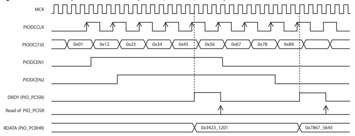
Figure 28-12. Parallel Capture Mode Waveforms (DSIZE=2, ALWYS=0, HALFS=1, FRSTS=0)
