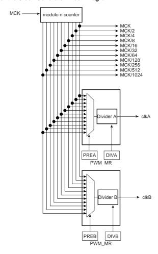
The PWM master clock (MCK) is divided in the clock generator module to provide different clocks available for all channels. Each channel can independently select one of the divided clocks.
