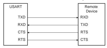
Setting the USART to operate with hardware handshaking is performed by writing the USART\_MODE field in the Mode Register (US\_MR) to the value 0x2.
