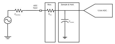
During the tracking phase the ADC needs to track the input signal during the tracking time shown below:
