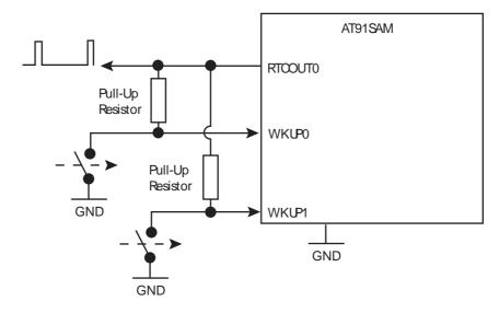
Figure 16-6. Low Power Debouncer (Push-to-Break switch, pull-down resistors)
