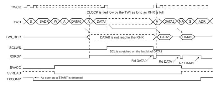
Notes: 1. At the end of the read sequence, TXCOMP is set after a STOP or after a REPEATED\_START + an address different from SADR.
