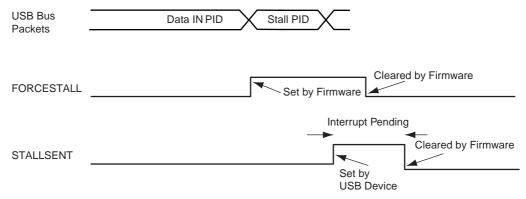
Figure 37-13. Stall Handshake (Data OUT Transfer)
