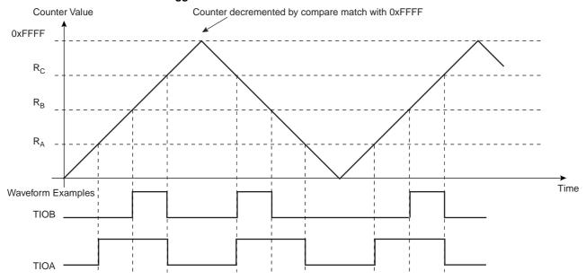
Figure 34-12. WAVSEL = 01 With Trigger
