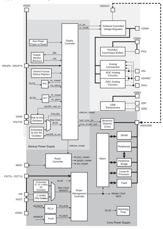
${\sf FSTT0-FSTT15} \ are possible \ {\sf Fast Startup Sources}, \ generated \ by \ WKUP0-WKUP15 \ Pins, but are not physical pins.$
