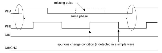
The direction change detection is disabled when QDTRANS is set to 1 in TC\_BMR. In this case the DIR flag report must not be used.
