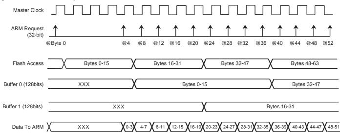
Note: When FWS is included between 1 and 3, in case of sequential reads, the first access takes (FWS+1) cycles, the other ones only 1 cycle.
