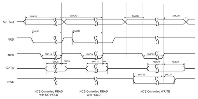
Figure 41-34. SMC Timings - NRD Controlled Read and NWE Controlled Write
