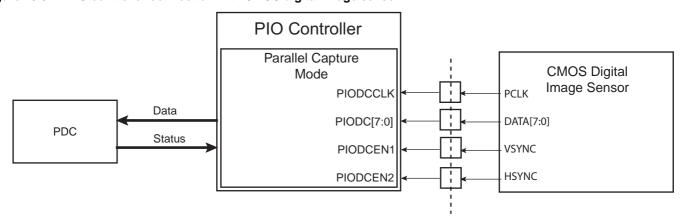
As soon as the parallel capture mode is enabled by writing the PCEN bit at 1 in PIO\_PCMR ("PIO Parallel Capture Mode Register"), the I/O lines connected to the sensor clock (PIODCCLK), the sensor data (PIODC[7:0]) and the sensor data enable signals (PIODCEN1 and PIODCEN2) are configured automatically as INPUTS. To know which I/O lines are associated with the sensor clock, the sensor data and the sensor data enable signals, refer to the I/O multiplexing table(s) in the product datasheet.
