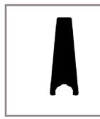
Spanners with notch for securing the notched nut
