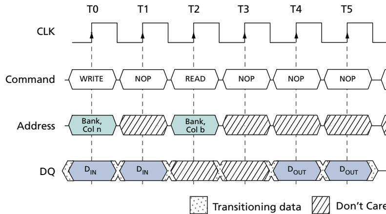
Note: 1. The WRITE command can be issued to any bank, and the READ command can be to any bank. DQM is LOW. CL = 2 for illustration.
