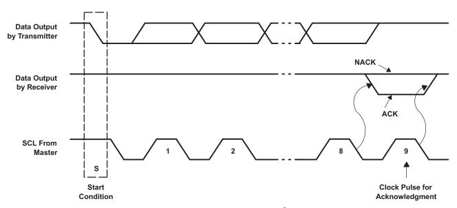
Figure 7. Acknowledgment on I<sup>2</sup>C Bus
