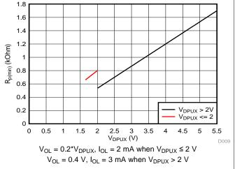
Figure 2. Minimum Pull-Up Resistance ( $R_{p(min)}$ ) vs Pull-Up Reference Voltage ( $V_{DPUX}$ )
