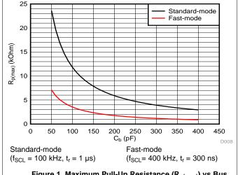
Figure 1. Maximum Pull-Up Resistance ( $R_{p(max)}$ ) vs Bus Capacitance ( $C_b$ )
