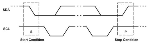
Figure 5. Definition of Start and Stop Conditions
