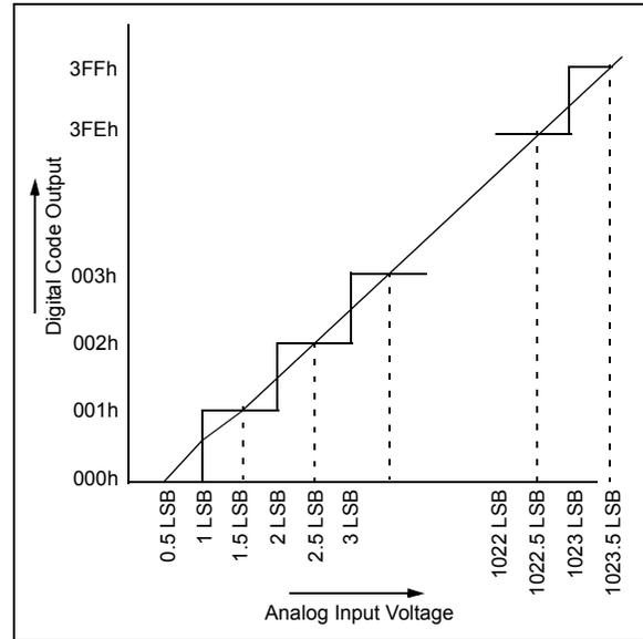
**FIGURE 18-3: ANALOG INPUT MODEL**
