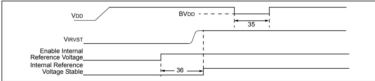
**TABLE 25-10: RESET, WATCHDOG TIMER, OSCILLATOR START-UP TIMER, POWER-UP TIMER AND BROWN-OUT RESET REQUIREMENTS**
