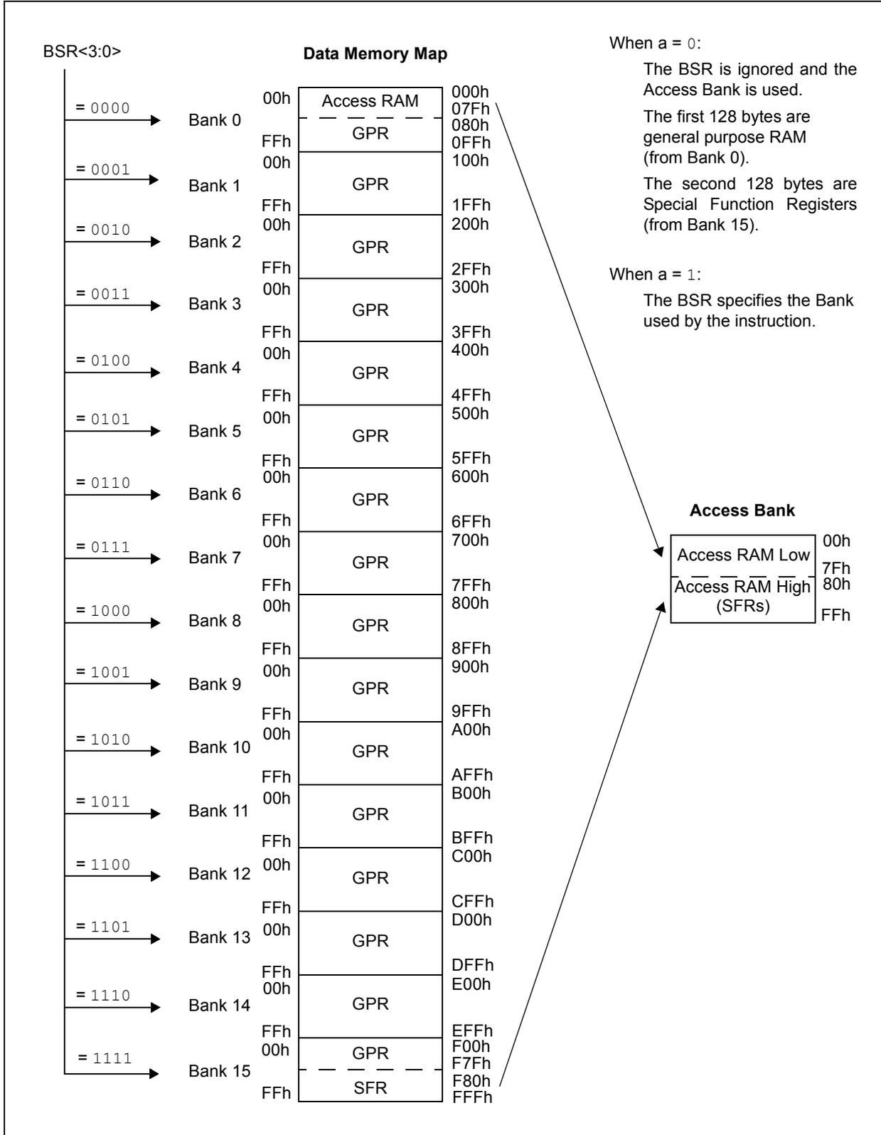
**FIGURE 5-8: USE OF THE BANK SELECT REGISTER (DIRECT ADDRESSING)**
