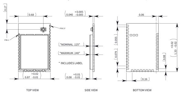
The following drawings show the standard (non-PRO) through-hole device.
