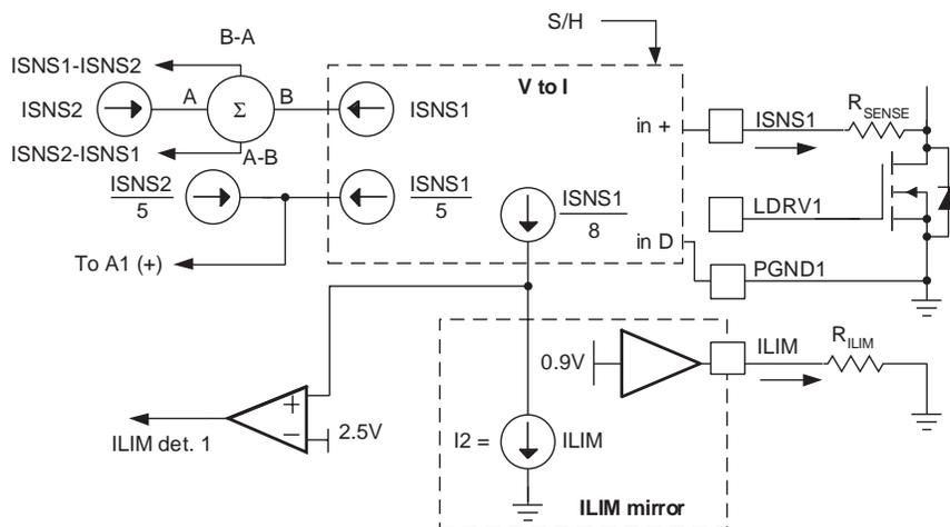
Figure 6. Current Limit and Active Droop Circuits
