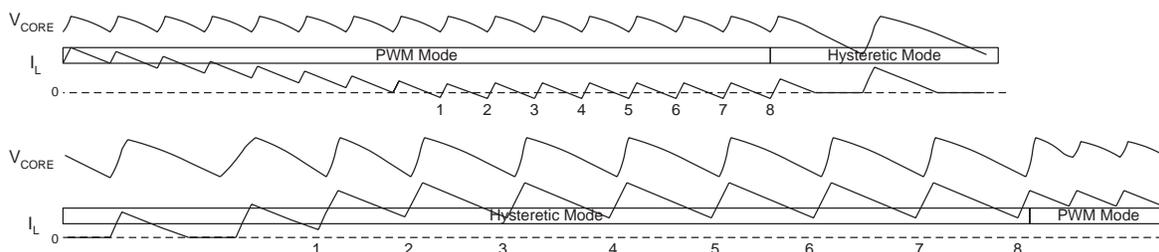
Figure 4. Transitioning between PWM and Hysteretic Mode
