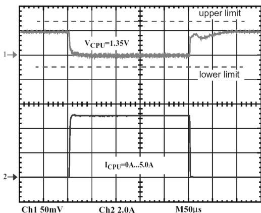
**Figure 8. Converter Response to 5A Load Step**
