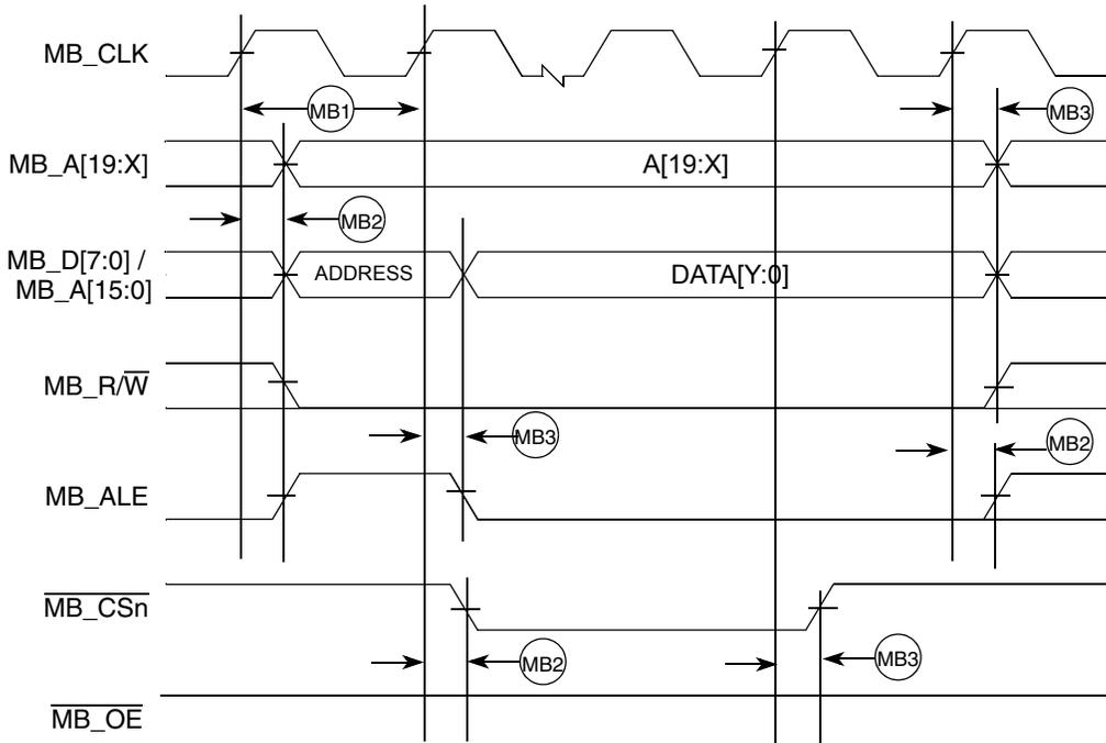
Figure 6. Mini-FlexBus Write Timing
