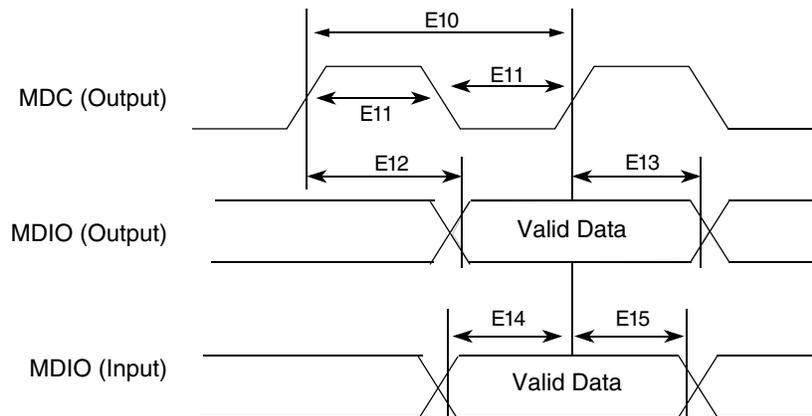
Figure 10. MII Serial Management Channel Timing Diagram
