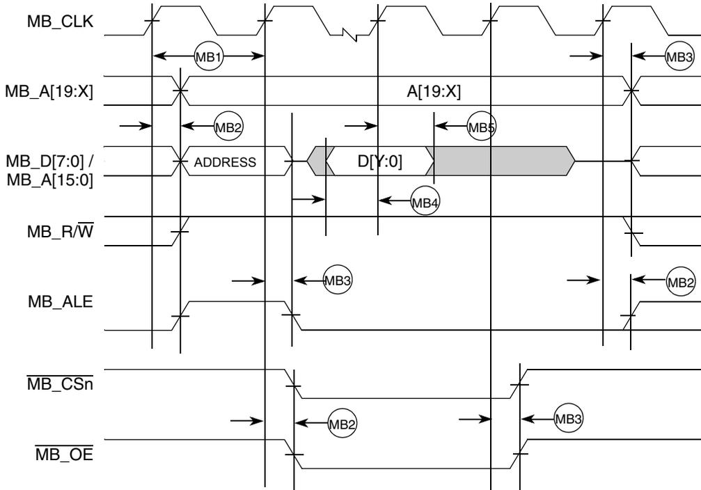
Figure 5. Mini-FlexBus Read Timing
