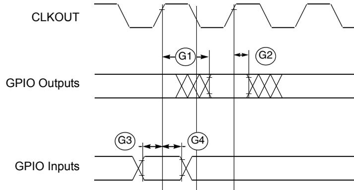
Figure 11. GPIO Timing
