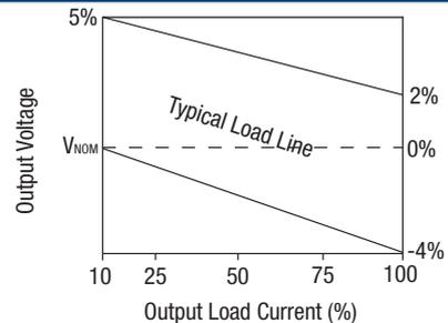
The voltage tolerance envelope shows typical load regulation characteristics for this product series. The tolerance envelope is the maximum output voltage variation due to changes in output loading.
