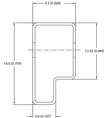
Unless otherwise specified all dimensions in mm [inches]  $\pm 0.55\text{mm}$  [0.022].
