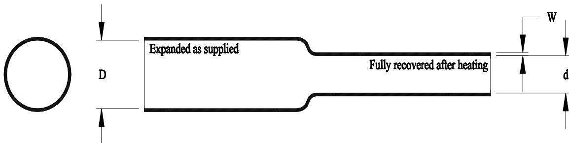
This specification covers the requirements for one type of single wall, electrical insulating, extruded tubing whose diameter will reduce to a predetermined size upon application of heat in excess of 140°C (284°F).
