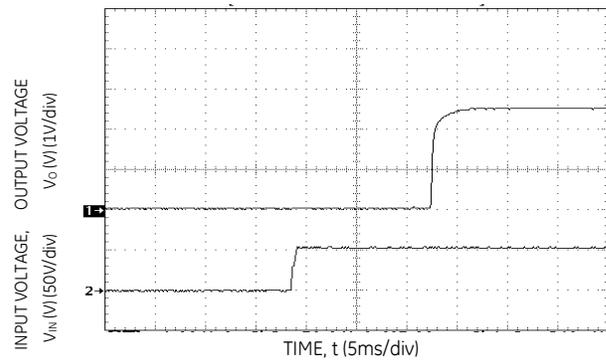
Figure 17. Typical Start-Up with application of Vin.
