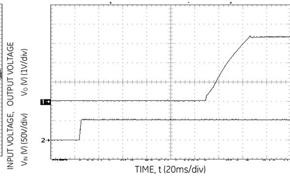
Figure 11. Typical Start-Up with application of Vin.
