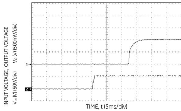
Figure 47. Typical Start-Up with application of  $V_{in}$ .
