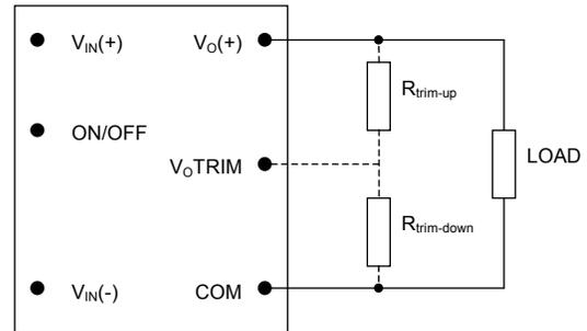
**Figure 65. Circuit Configuration to Trim Output Voltage.**
