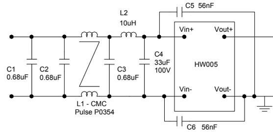
Figure 67. Suggested Configuration for EN55022 Class B.
