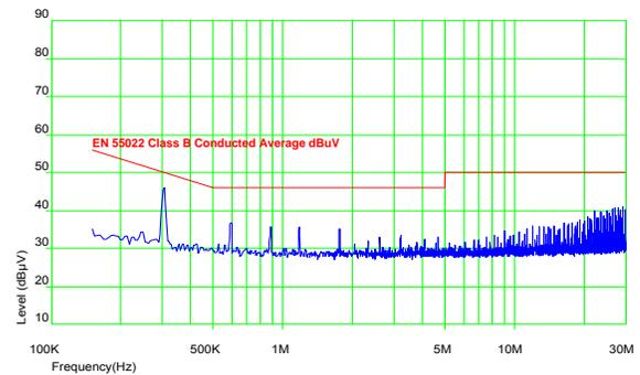
Figure 68. EMC signature using above filter, HW005A0F.
