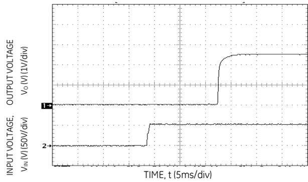
Figure 17. Typical Start-Up with application of Vin.
