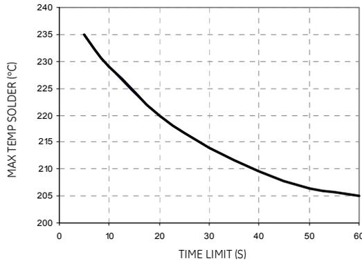
Figure 73. Time Limit Curve Above 205°C Reflow .
