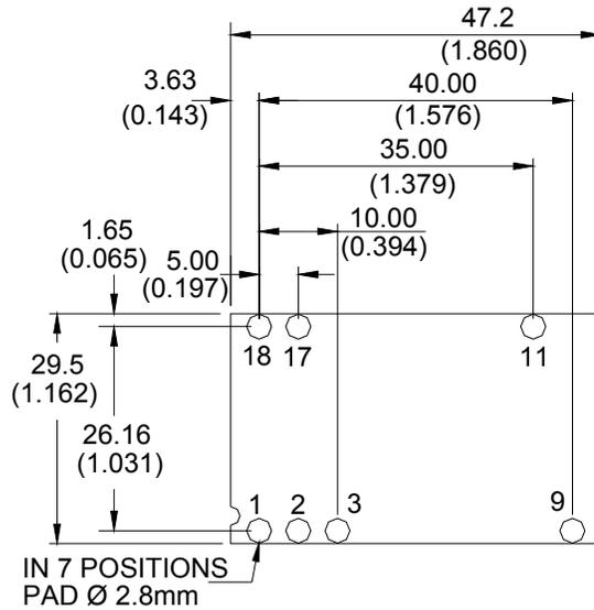
Surface Mount Pad Layout – Component side view
