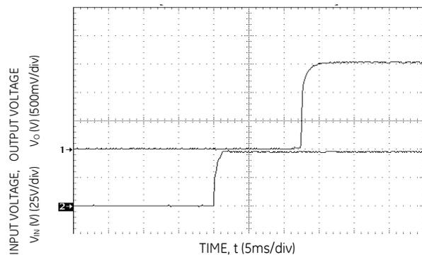
Figure 35. Typical Start-Up with application of Vin.
