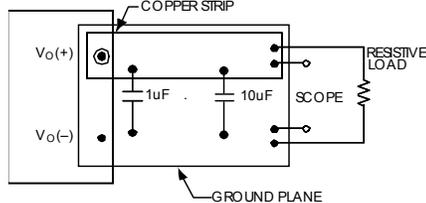
NOTE: All voltage measurements to be taken at the module terminals, as shown above. If sockets are used then Kelvin connections are required at the module terminals to avoid measurement errors due to socket contact resistance.
