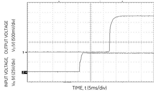
Figure 29. Typical Start-Up with application of Vin.
