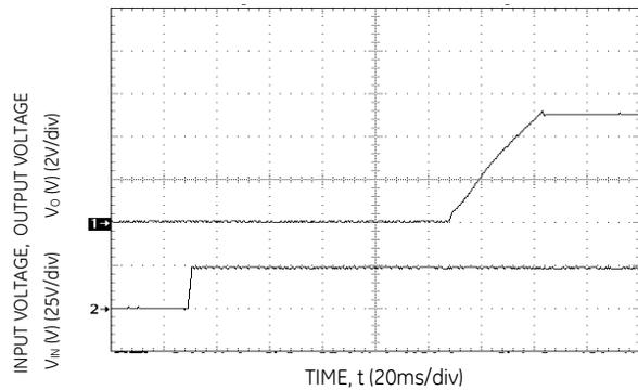
Figure 53. Typical Start-Up with application of Vin.
