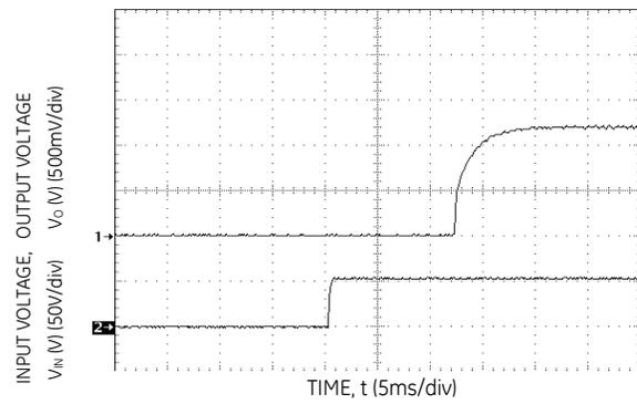
Figure 41. Typical Start-Up with application of Vin.
