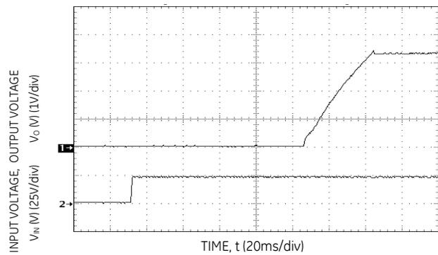
Figure 59. Typical Start-Up with application of Vin.
