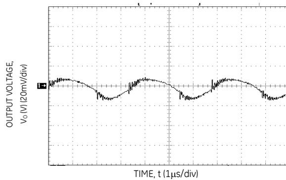
Figure 2. Typical Output Ripple and Noise.
