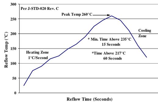
Figure 74. Recommended linear reflow profile using Sn/Ag/Cu solder.
