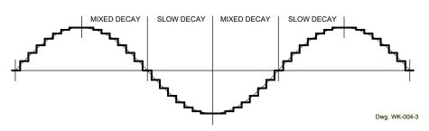
Figure 5 — Microstepping/Sinusoidal Drive Current
