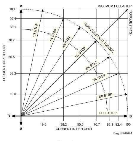
Figure 5 — Current and Displacement Vectors
