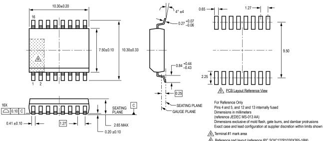
Alformatic Reference pad layout (reference IPC SOIC127P1030X265-16M) All pads a minimum of 0.20 mm from all adjacent pads; adjust as necessary to meet application process requirements and PCB layout tolerances
