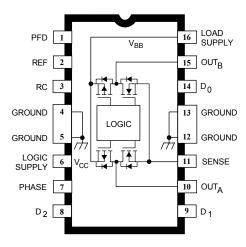
Note the A4975SB (DIP) and the A4975SLB (SOIC) are electrically identical and share a common terminal number assignment.
