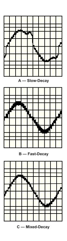
Figure 3 — Sinusoidal Drive Currents
