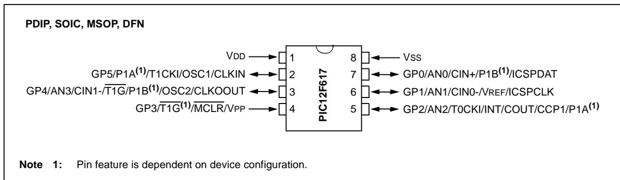
**TABLE 2: PIC12F617 PIN SUMMARY (PDIP, SOIC, MSOP, DFN)**
