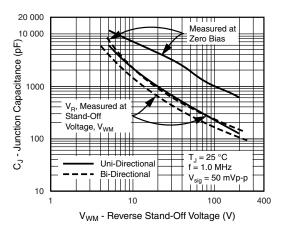
Fig. 4 - Typical Junction Capacitance Uni-Directional
