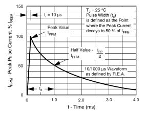
Fig. 3 - Pulse Waveform
