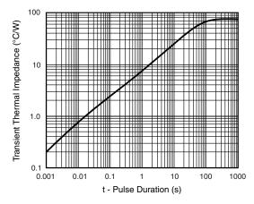
Fig. 5 - Typical Transient Thermal Impedance
