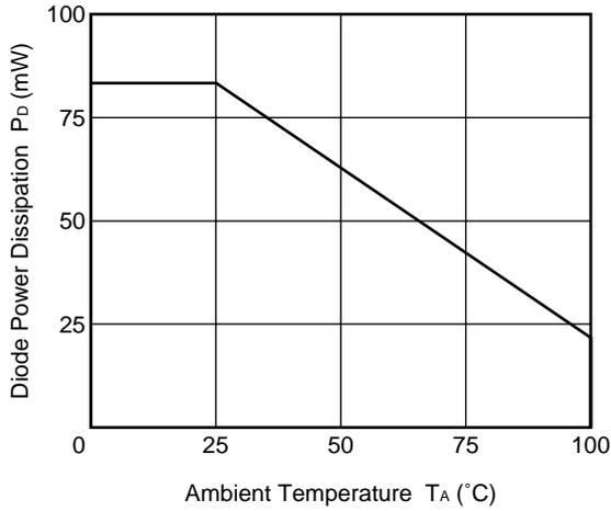
TRANSISTOR POWER DISSIPATION vs. AMBIENT TEMPERATURE
