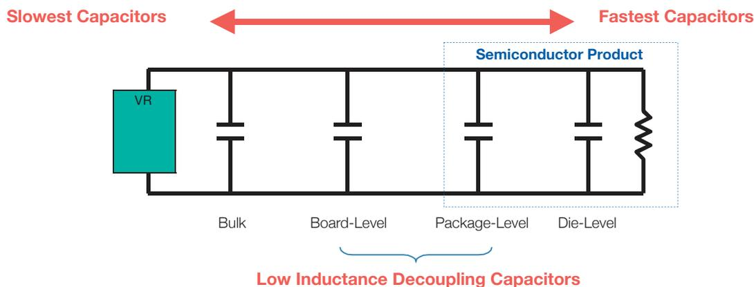
Figure 1 Classic Power Delivery Network (PDN) Architecture
