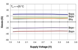
Switch Points vs Supply Voltage
