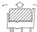
4. In case there is not enough space to grasp relay with fingers, use screwdrivers in the way shown below.
