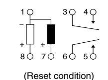
Since this is a polarized relay, the connection to the coil should be done according to the above schematic.
